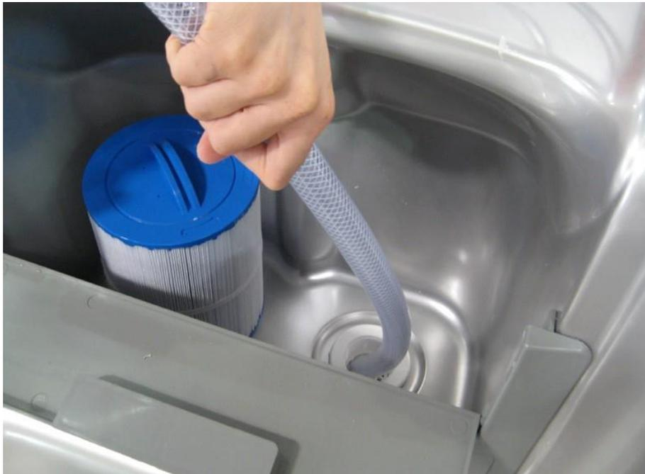
Figure 10. Filling Location in Filter Housing
