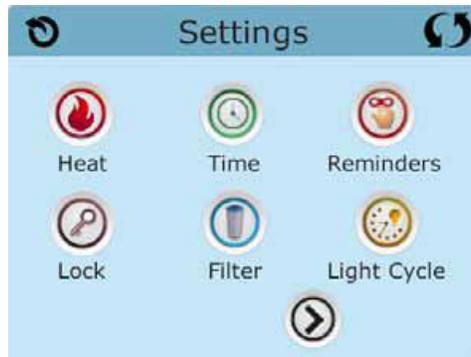
The Heat Icon
